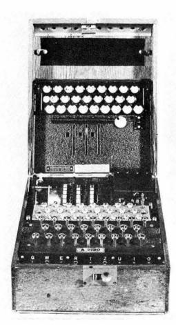
THE FAMOUS GERMAN ENIGMA coding machine is based on a computationally difficult problem, but the Germans failed to anticipate the electronic computer. The English developed a computer and put the first one, Colossus, into operation in 1943 specifically to work on Enigma ciphers. The millions of computations required to decode Enigma messages were performed in hours. The same calculations, made by hand, would have taken a thousand years.
